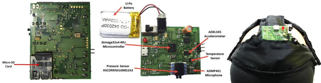
Fig. 1. ARAM's Custom built PCBs. (Left) Back of the PCB including the MicroSD card slot. (Middle) Front of the PCB including all sensors and battery. (Right) The entire circuit was housed inside the cloth pocket at the top of the ARAM mask.
