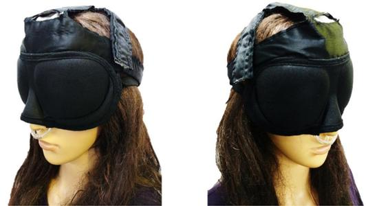
Fig. 2. ARAM's cloth housing including Velcro straps around the patient's head. The device is designed to look and feel like a sleep mask so as to simplify installation for the patient, while still offering secure support for the sensors and cannula.
