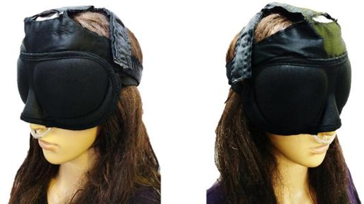
Fig. 2. ARAM's cloth housing including Velcro straps around the patient's head. The device is designed to look and feel like a sleep mask so as to simplify installation for the patient, while still offering secure support for the sensors and cannula.
